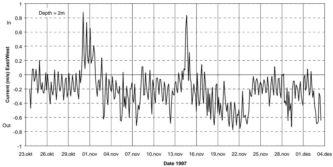
**Figure 34.** East/West current (m/s) at 2 m depth inside Svinesund (station D), as measured by the ADP.
