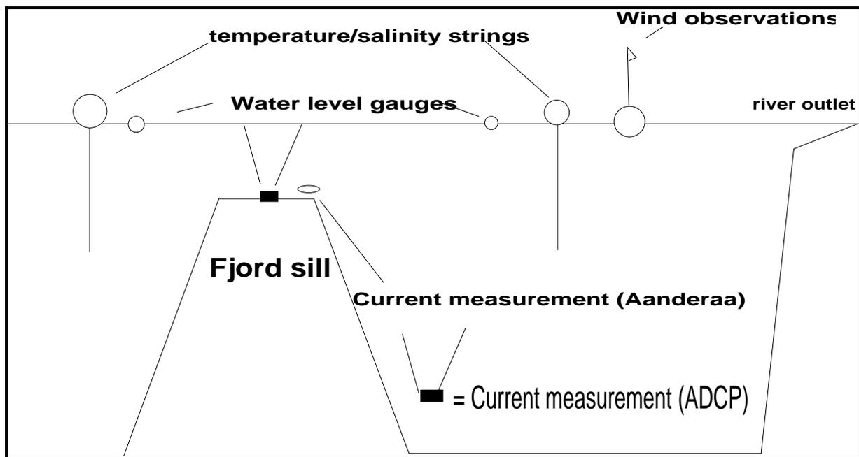
**Figure 3.** Principal instrument deployment in the fjords.
