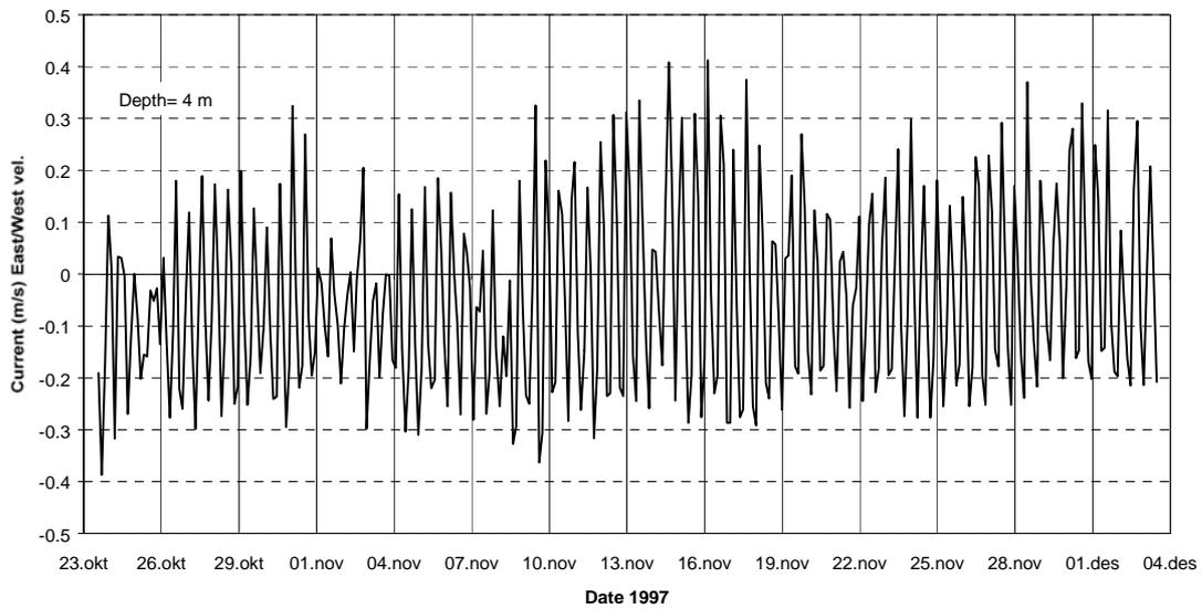
**Figure 35.** East/West current (m/s) at 4 m depth inside Svinesund (station D), as measured by the ADP.
