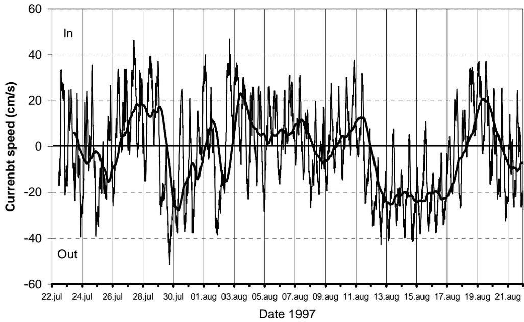
**Figure 11.** Current speed (cm/s) at 27 m depth in the Brevikstrømmen, projected on a 280 (positive) - 100 degree axis. The figure also includes the 25-hours sliding mean.
