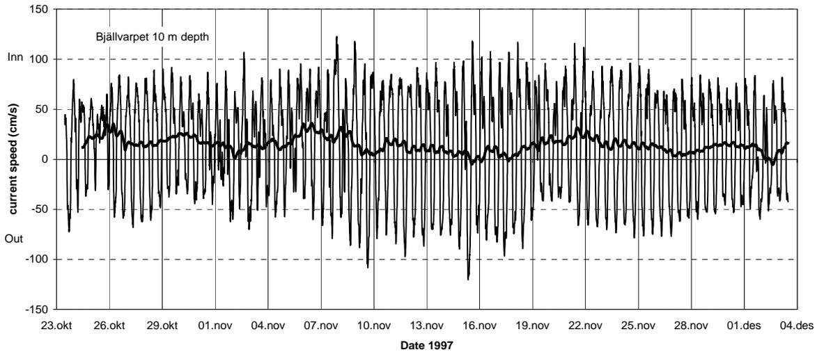
**Figure 28.** Current (in/out) at 10 m depth, Bjällvarpet (station A).
