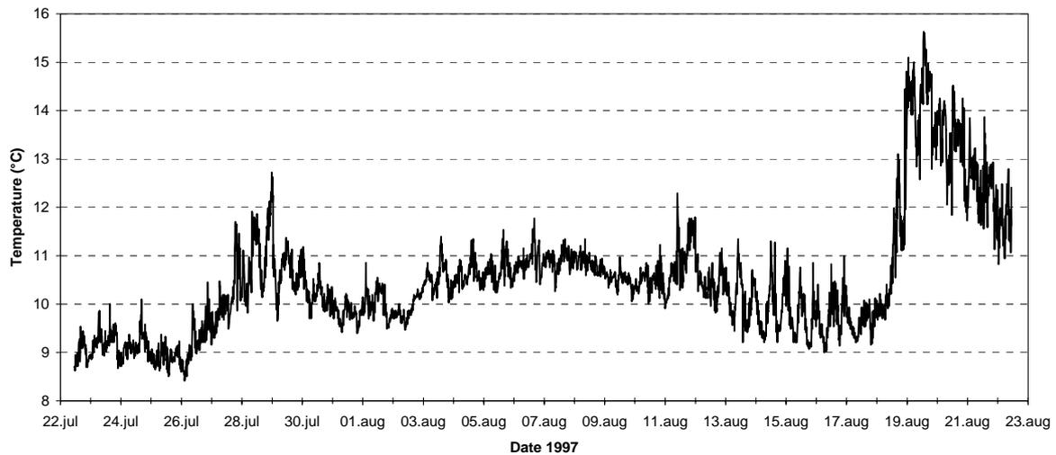
**Figure 10.** Temperature (°C) at 27 m depth in the Brevikstrøm, July-August 1997, in the sill area.
