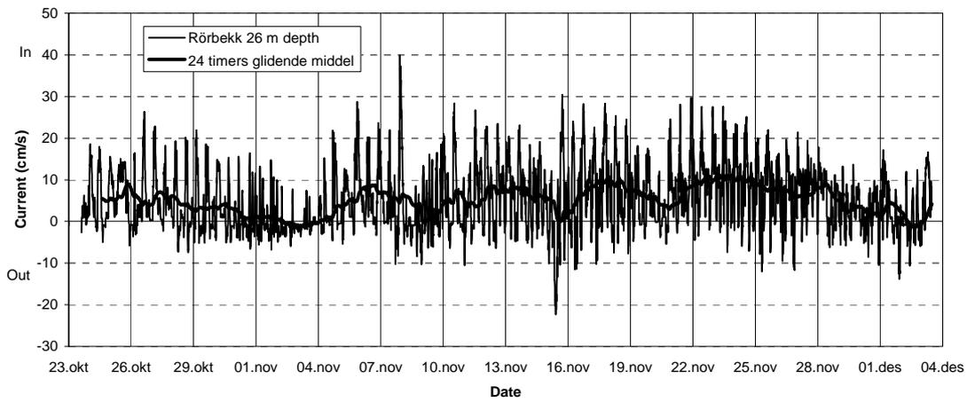
Figure 32. Current (in/out) at 26 m depth, Rørbekk (station B).
