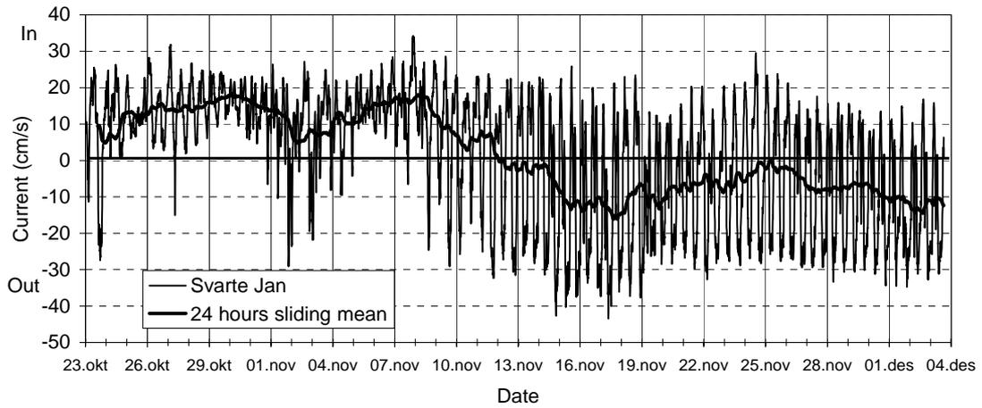
**Figure 42.** Current (in/out) at 18 m depth, Svarte Jan (station H).
